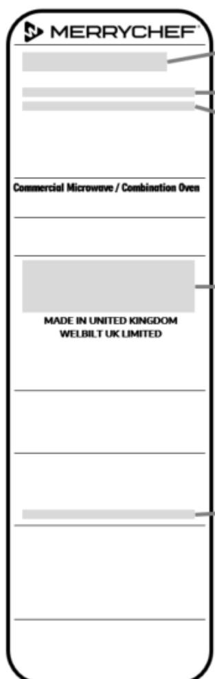
The diagram shows the back panel of a MERRYCHEF microwave oven. Callout 1 points to the model number 'eikon e2s'. Callout 2 points to the product code 'D'. Callout 3 points to the power options 'F', 'G', and 'B'. Callout 4 points to the voltage options '30', 'MV5', 'MV6', and '00'. Callout 5 points to the serial number '1, 2, ...'. The technical data label also includes information about frequency, output, information exchange, and region.
