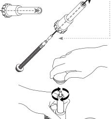
**INSTALL LARGE O-RING** into valve body. Apply food equipment lubricant on o-ring.
