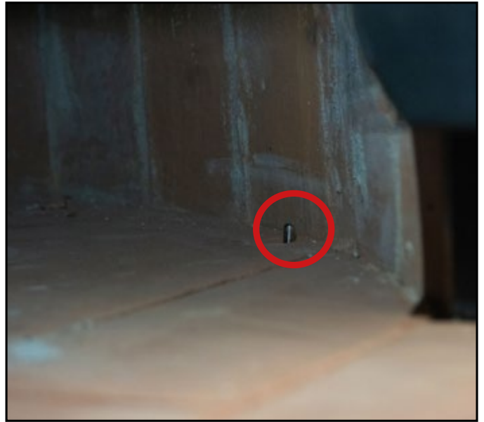
5 - Insert the probe into the hole so that it protrudes 1cm on the refractory surface.
