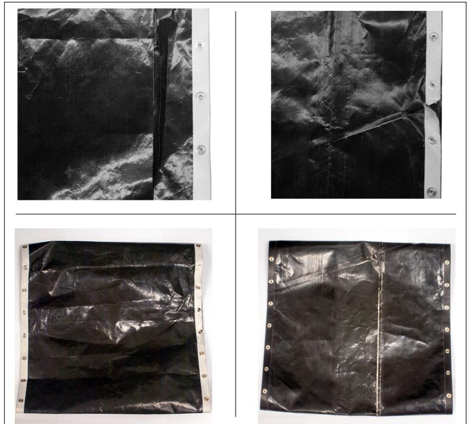
Figure 6. Examples of Damaged Belt Wraps
