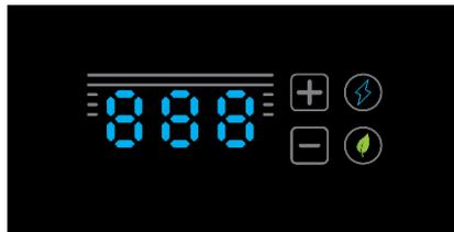
At factory settings, the appliance starts at 60°C but stores the programmed temperature setting when power is cut.
