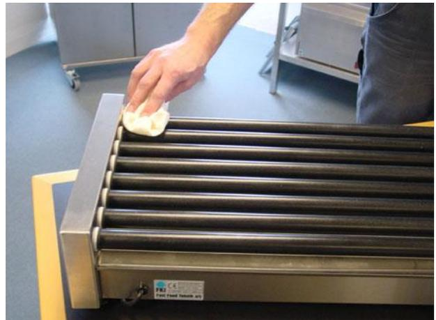
Wipe the rollers with a damp cloth soaked in detergent. Dry inwards towards the centre of the rollers to prevent grease/fat from being pushed back into the cabinet.
