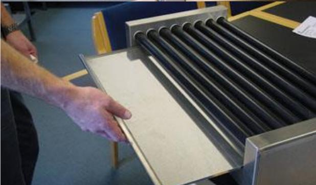
Remove the tray under the rollers and clean it.
