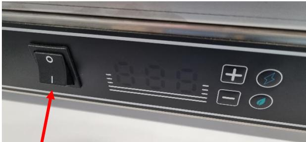
Turn on the roller grill and set the temperature to the lowest setting. This causes the rollers to turn and makes them easier to
