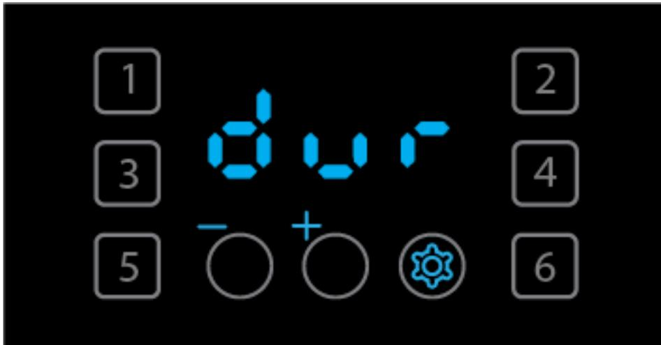
Figure 9, setting the duration of the buzzer sound.
