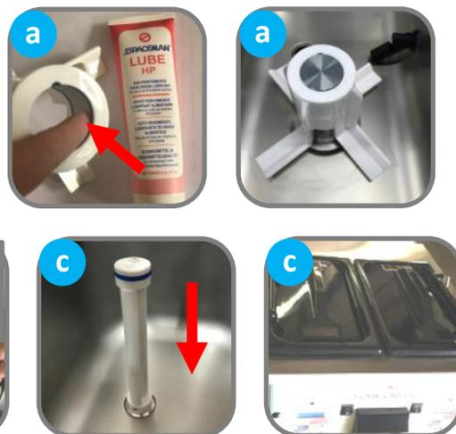
**IMPORTANT:** After sanitizing the machine, **DO NOT** rinse or touch areas that have been sanitized. Product must be added immediately. If new product will not be added immediately, rinse machine with clean water and loosen door hand-screws to allow cylinders to air-dry. Sanitize machine before using again.
