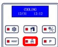
Turn on freezing immediately to cool product down to serving consistency. Use when quick serve is required after long idle period.
