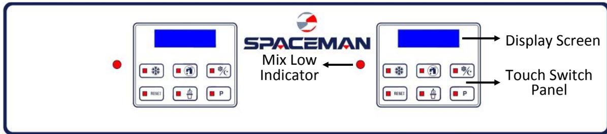
**MIX LOW INDICATOR:** A mix level indicating light is located at the front of the machine. When the light is "ON", it indicates that the mix hopper has a low supply of mix and should be refilled as soon as possible. Always maintain at least 2cm of mix in the hopper. If you neglect to add mix, a freeze-up may occur. This will cause eventual damage to the beater assembly, the dispensing door, and gear box.
