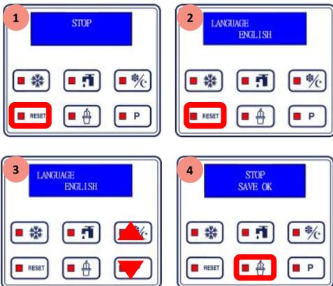
1. Press RESET to stop machine functions. Press and hold RESET until display shows settings.
