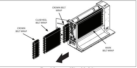
Figure 5. Remove and Discard the Belts DO NOT REUSE THE BELTS!
