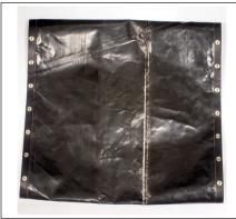
Belt is damaged and folded. **Replace Belt.**
