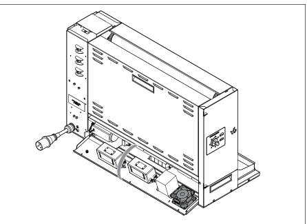
Figure 7. Accessing Rear Cooling Fan
