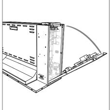
Figure 6. Accessing Top Cooling Fan
