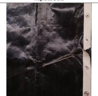
Belt is missing snaps and is damaged. Replace Belt.
