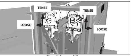
**Figure 3. Conveyor Rollers**
