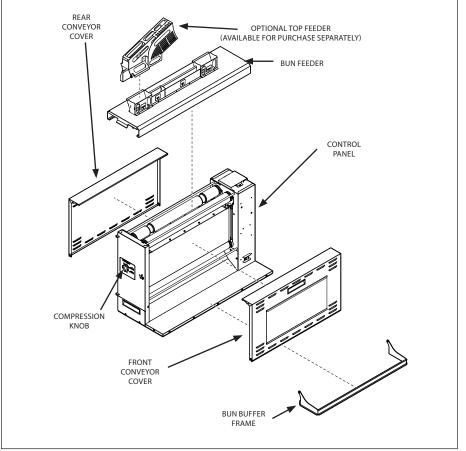
Figure 1. GST-5V Components (Belts not Shown)
