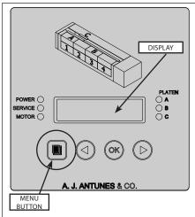
Figure 2. GST-5V Control Panel and Display
